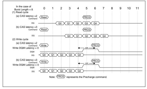
11.23 CKE/DQM Input Timing (Write Cycle)
