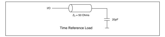
Input signal transition time between VIH and VIL is assumed as 1 Volts/nS.
